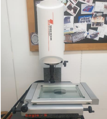
Mold shape measurement using microscope
